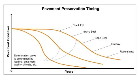
Optimum maintenance timing is critical to preserving your pavement investment. The more deteriorated the pavement, the greater the treatment cost.
